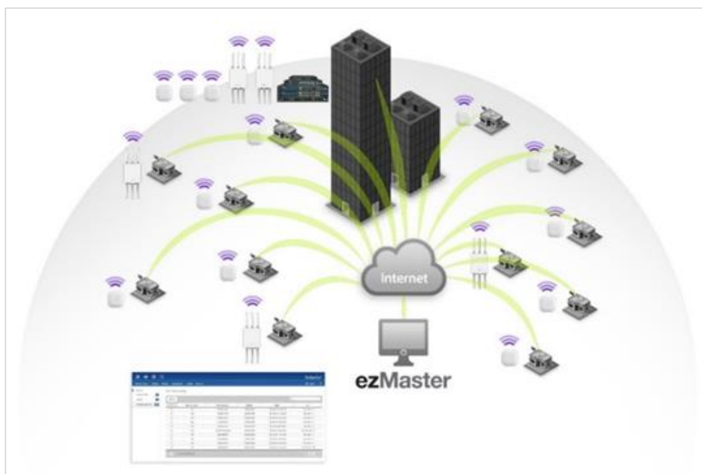
Figure 9 – Centralized Management Architecture
