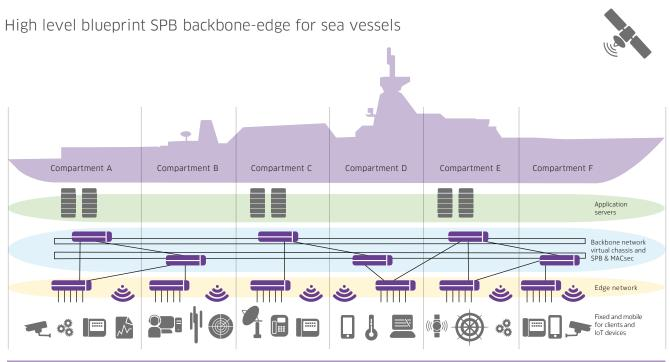
IS-IS SPB and MACsec, two protocols combined to build a highly resilient, scalable and secured network
